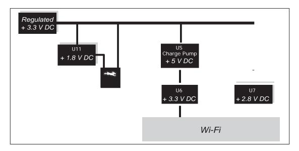
Figure F-2. RCM5600W/ RCM6600W Onboard Power Supplies
