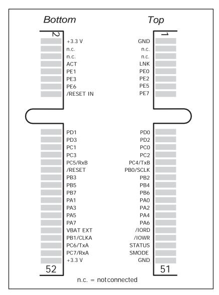
Figure 9. RCM5600W Pinouts
