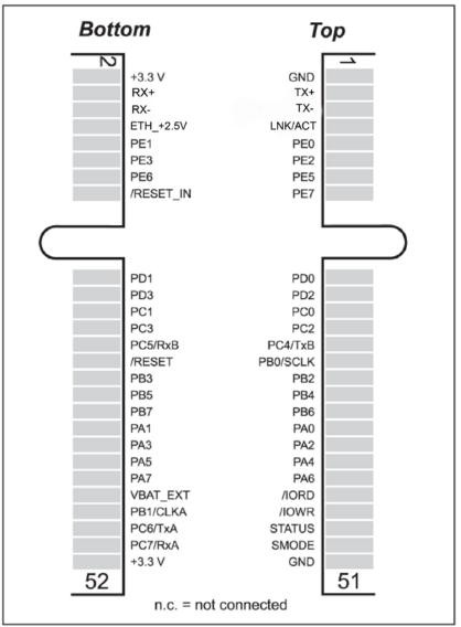
Figure 10 shows the RCM6600W pinouts for the edge connector.
