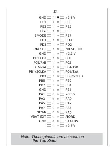
Figure D-4. MiniCore Boards Pinout
