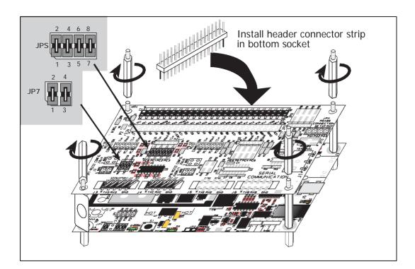
Figure 17. Install Serial Communication Accessory Board
