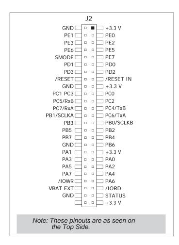
Figure B-5. Interface Board Pinout
