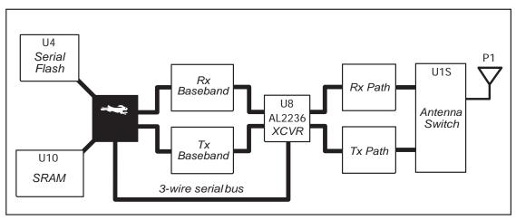
Figure 13. RCM5600W/RCM6600W Wi-Fi Block Diagram
