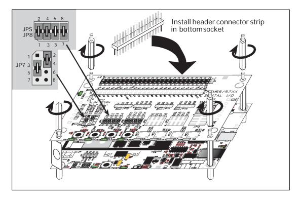
Figure 16. Install Digital I/O Accessory Board
