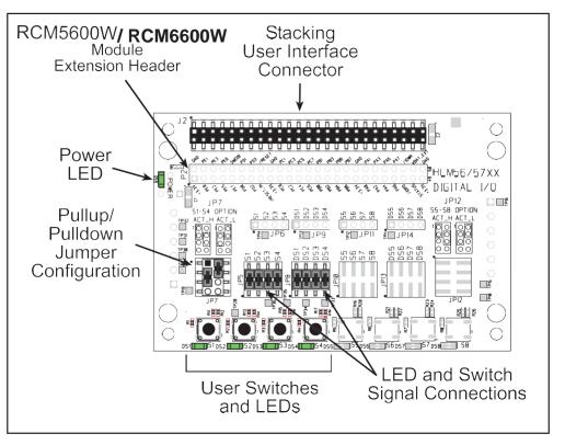
Figure D-1. Digital I/O Accessory Board
