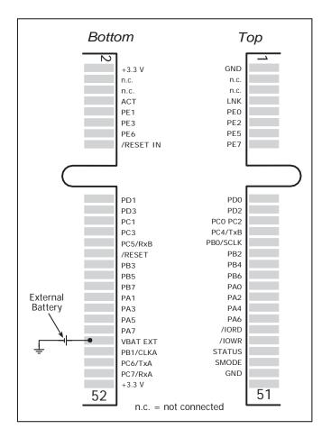
Figure F-1. External Battery Connections
