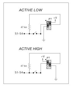
Figure D-5. Pushbutton Switch Configuration
