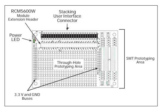
Figure C-1. Prototyping Board
