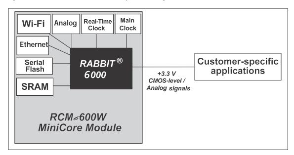
Figure 8. RCM6600W Subsystems
