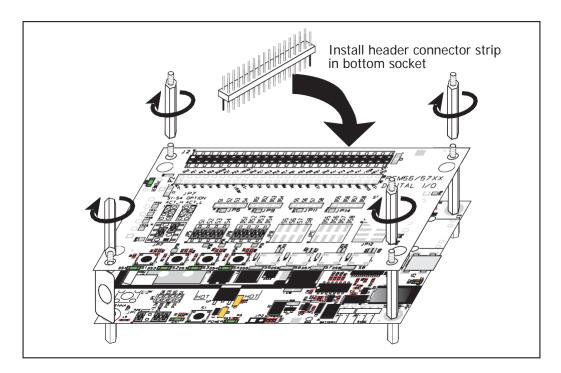
Figure D-7. Install Additional Boards
