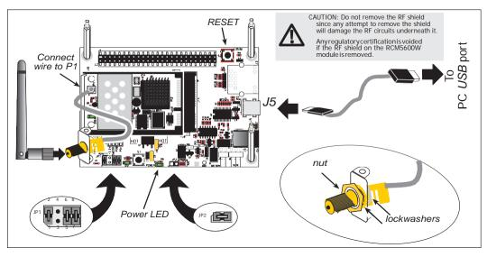
Figure 4. Connect Antenna and USB Cable
