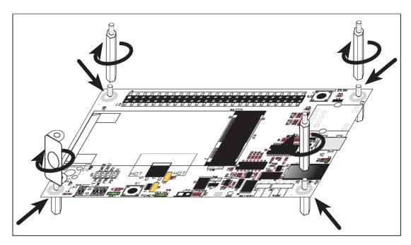
Figure 2. Insert Standoffs/Connectors
