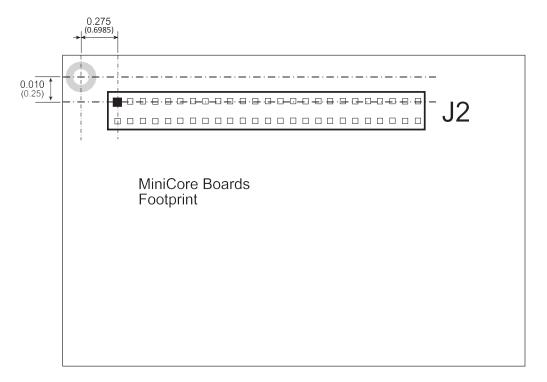
Figure B-3. Interface Board Footprint
