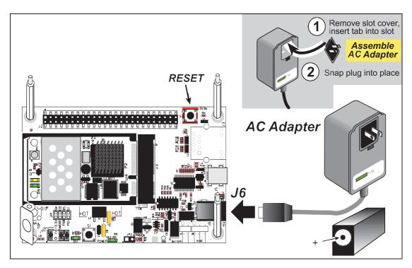
Figure 5. Alternate Power Supply Connections—Deluxe Development Kit
