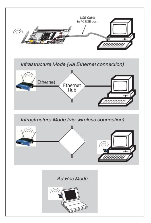
Figure 15. Wi-Fi Host Setup
