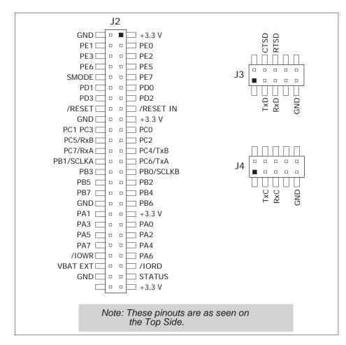
Figure E-4. Serial Communication Accessory Board Pinout
