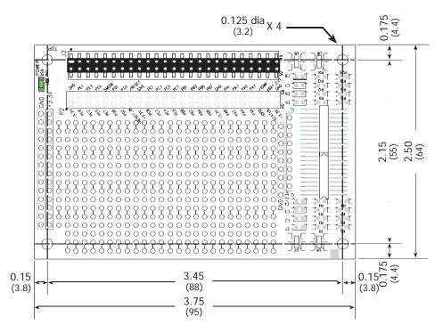
Figure C-2. Prototyping Board Dimensions
