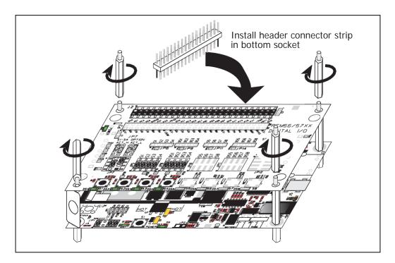
Figure E-6. Install Additional Boards
