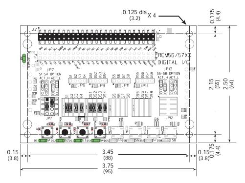
Figure D-2. Digital I/O Accessory Board Dimensions
