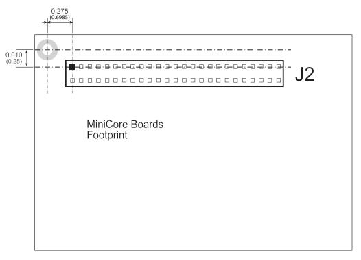
Figure D-3. MiniCore Boards Footprint
