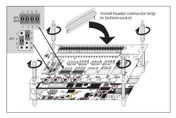
Figure 6. Install Digital I/O Accessory Board
