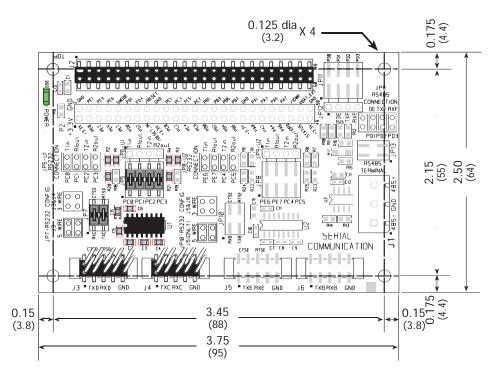
Figure E-2. Serial Communication Accessory Board Dimensions
