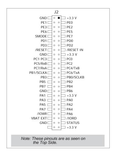
Figure C-4. MiniCore Boards Pinout
