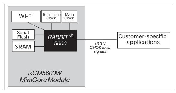
Figure 7 shows the Rabbit-based subsystems designed into the RCM5600W.
