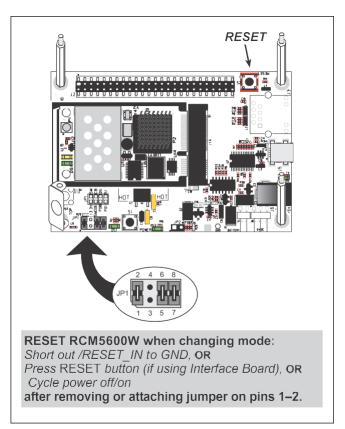
Figure 14. Switching Between Program Mode and Run Mode
