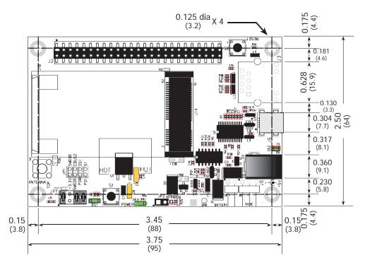
Figure B-2. Interface Board Dimensions
