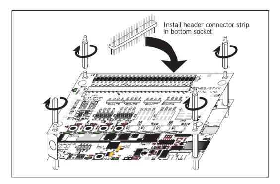
Figure C-5. Install Additional Boards
