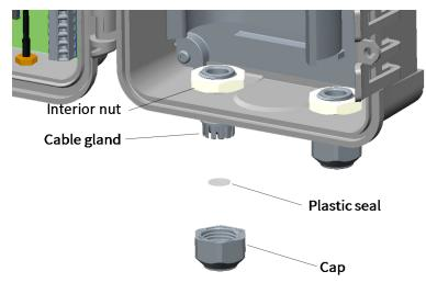
2. Unscrew the gland cap and remove the plastic seal.
