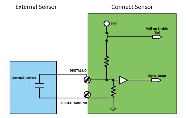
The following figure shows a digital input with the pull-up resistor disabled.
