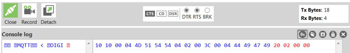
You can verify the response from the broker as a CONNACK by comparing it to the structure of a CONNACK packet in the MQTT documentation, which is available at [http://docs.oasis-open.org/mqtt/mqtt/v3.1.1/os/mqtt-v3.1.1-os.html#\\_Toc398718081](http://docs.oasis-open.org/mqtt/mqtt/v3.1.1/os/mqtt-v3.1.1-os.html#_Toc398718081).
