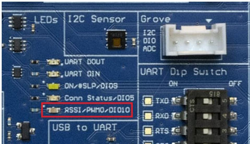
1. Note the **DIO10** LED on the XBIB board. The following image highlights it in a red box. The LED is normally off.
