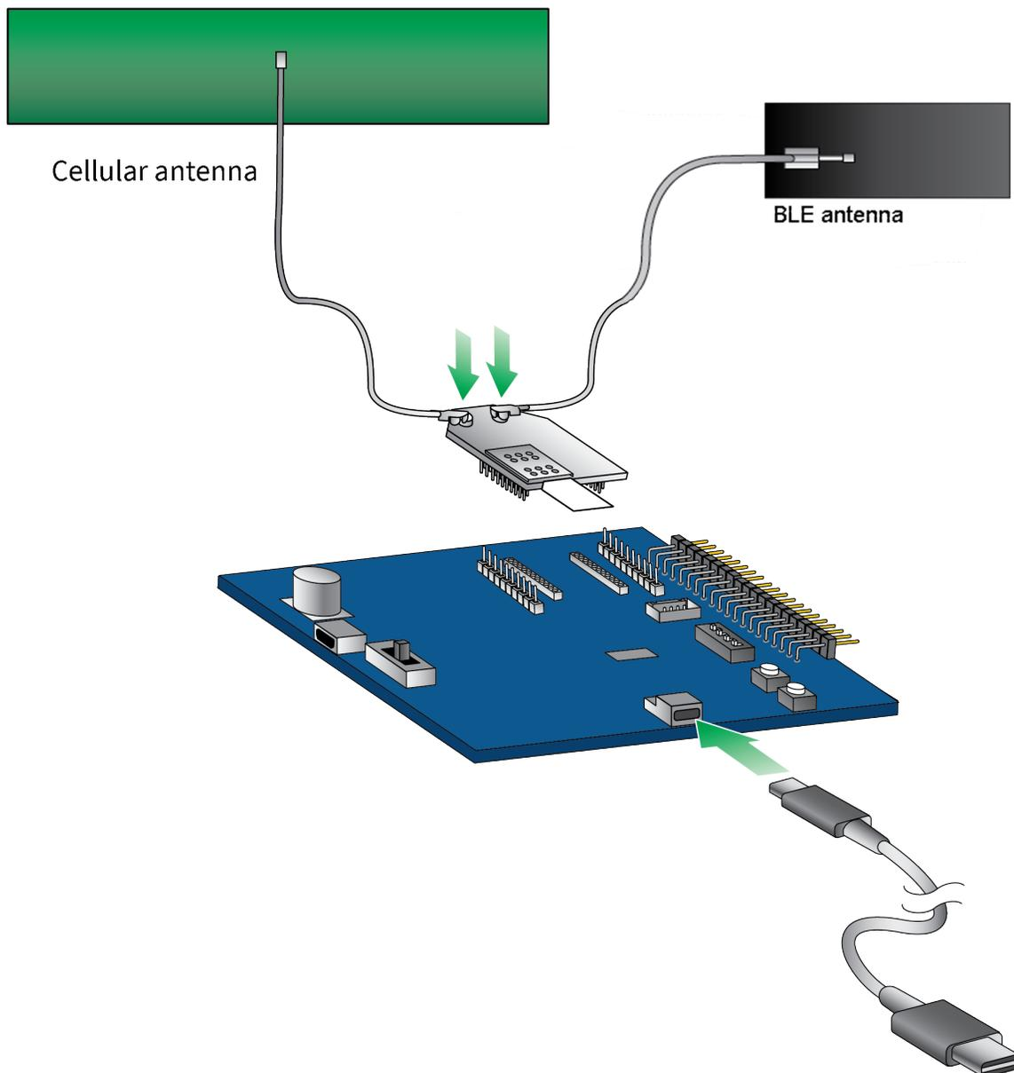
1. The XBee Smart Modem should already be plugged into the development board. For more information about development boards, see [Development boards](#).
