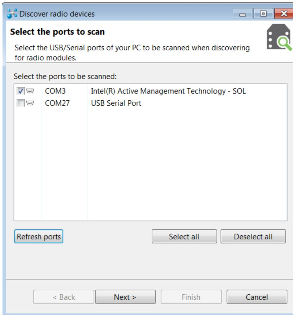
4. Remove the development board from the USB port and view which port name no longer appears in the **Discover radio devices** list of ports. The port name that no longer appears is the correct port for the development board.
