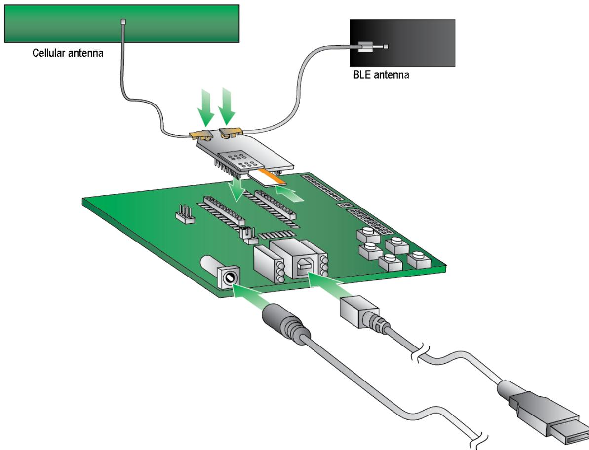
1. The XBee Smart Modem should already be plugged into the development board. For more information about development boards, see [Development boards](#).
