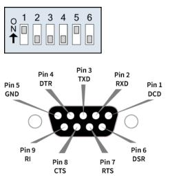
The following table provides the RS-232 signals and their implementations on the Module Assembly. Low-asserted signals have a horizontal line over the pin name.
