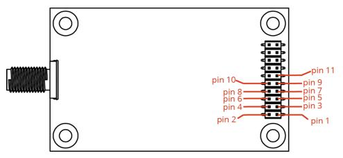
When integrating the module with a Host PC board, leave all lines that you do not use disconnected (floating).
