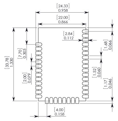
While the underside of the module is mostly coated with solder resist, we recommend that the copper layer directly below the module be left open to avoid unintended contacts. Copper or vias must not interfere with the three exposed RF test points on the bottom of the module (see below). Furthermore, these modules have a ground plane in the middle on the back side for shielding purposes, which can be affected by copper traces directly below the module.
