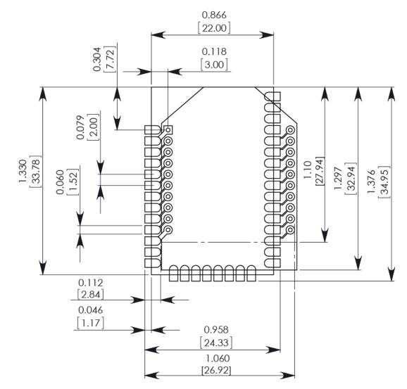
The round holes in the diagram are for the through-hole design, and the semi-oval pads are for the surface-mount design. Pin 1 of the through-hole design lines up with pad 1 of the surface-mount design, but the pins are actually offset by one pad—see Pin mapping. By using diagonal traces to connect the appropriate pins, the layout works for both modules.
