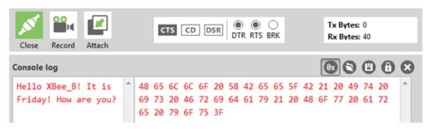
6. In the Console log area for XBEE\_B, type "Hello XBee\_A! It is Friday! How are you?"
