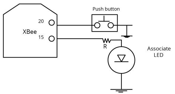
A pushbutton and an LED can be connected to the XBee 868LP RF Module pins 33 and 28 (SMT), or pins 20 and 15 (TH) respectively to support the commissioning pushbutton and associate LED functionalities.
