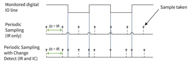
Enabling edge detection forces an immediate sample of all monitored digital I/O lines if any digital I/O lines change state.
