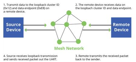
The configuration steps to send data to the loopback cluster ID depend on the AP setting.
