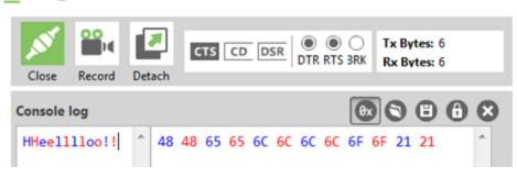
**Tip** Use the **Send a single packet** command to send and have an entire message loop back, instead of having individual characters loop back. To do this, click the **Add new packet** button
