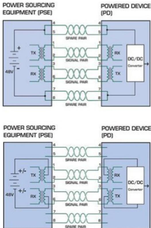
The power provided with powered Ethernet is nominally 48 volts at a maximum of 350 mA or about 13 watts. 1500V isolation is also provided for safety.
