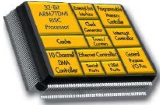
**The NetSilicon NS7520 from Digi International is a 32-bit RISC processor that features an ARM core with internal memory, DMA, Ethernet, serial and bus controllers.**
