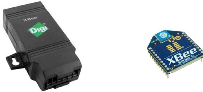
Depending on the preferred method of deployment, external or embedded solutions are available. External adapters can connect to a device's native serial port or to an analog or digital output from the device, or a module can be integrated into the device. These options are available in the same form factors regardless of the type of RF communication chosen.
