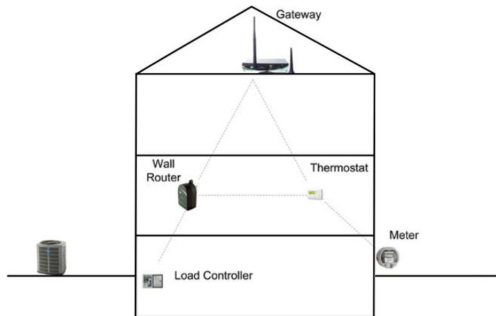
In the first diagram, the gateway is located to provide effective communications to the various endpoint devices and to the uplink network. A ZigBee wall router is placed to provide additional coverage where needed.
