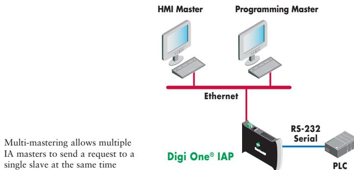
Multi-mastering allows multiple IA masters to send a request to a single slave at the same time
