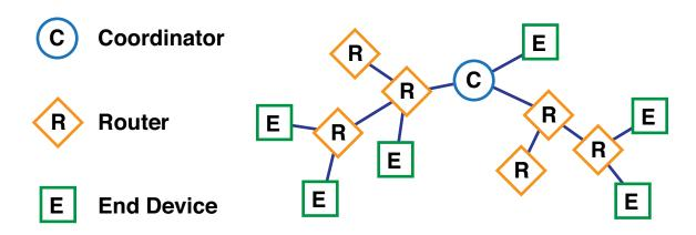
Coordinators are the most capable of the three node types. There is exactly one coordinator in each network and it is the device that establishes the network originally. It is able to store information about the network, including security keys.
