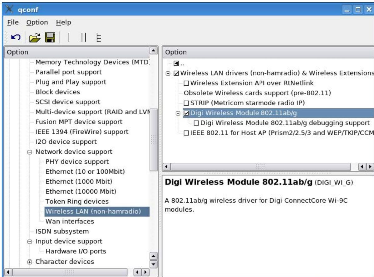
The wireless driver support is included by selecting the **Digi Wireless Module 802.11 ab/g** component.
