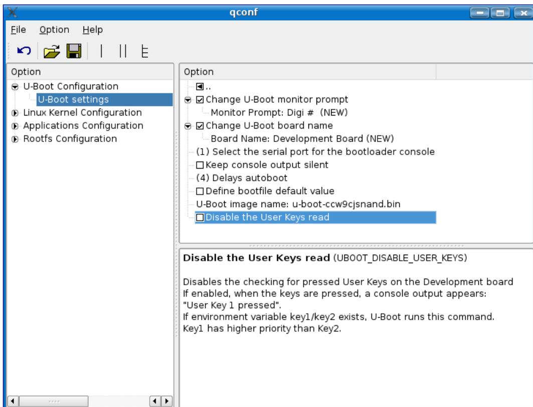
In the U-Boot configuration tool, selecting **U-Boot Configuration > U-Boot settings** displays several U-Boot configuration settings:
