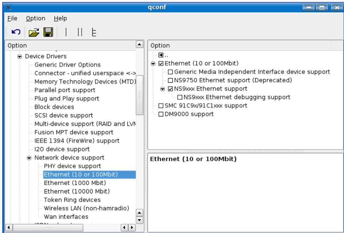
The Ethernet driver support is included by checking the **NS9xxx Ethernet support** component.
