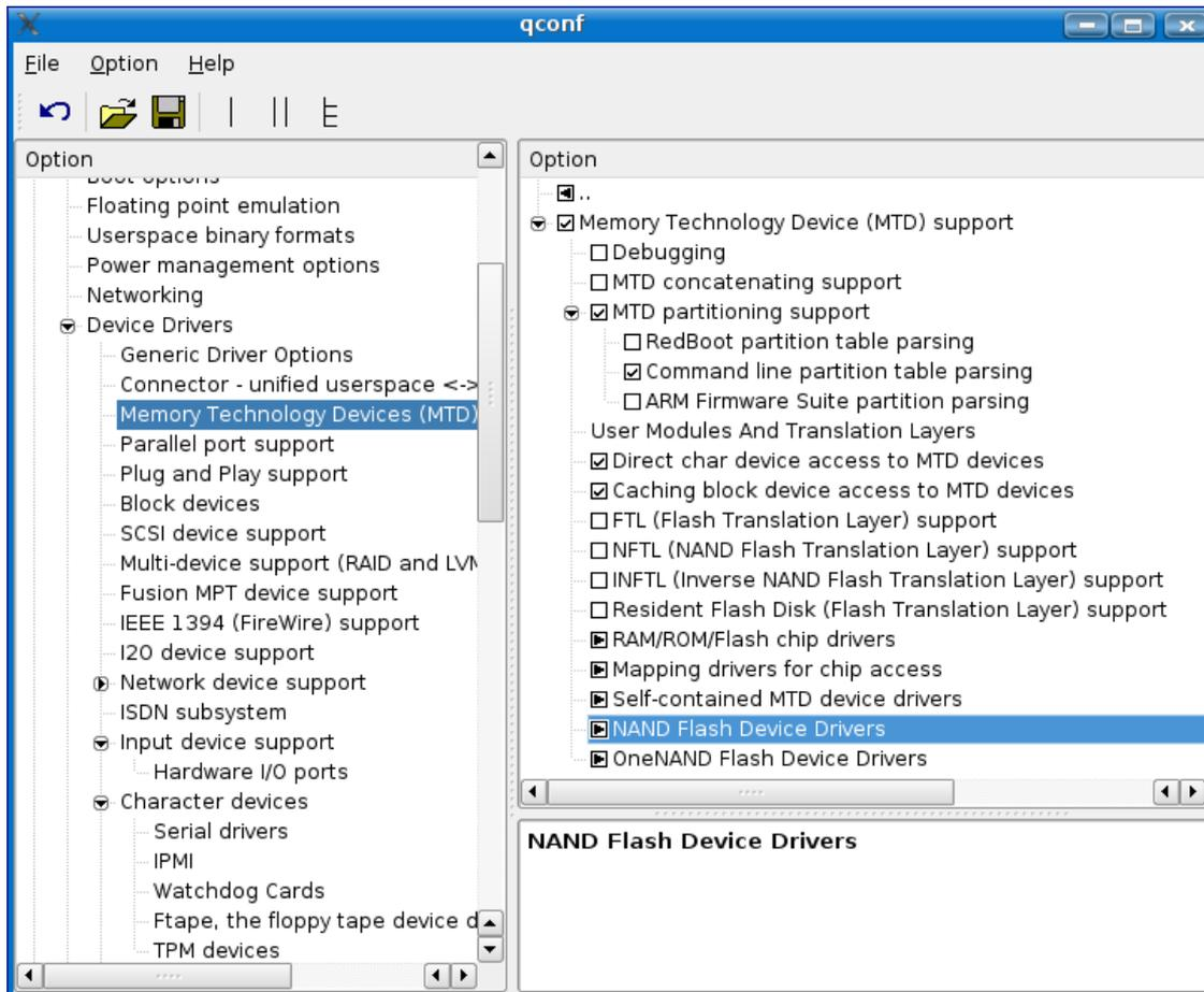
To support the Flash memory device in Linux, include support for Memory Technology Devices (MTD) and partitioning. The specific driver is included in the **NAND Flash Device Drivers**. To access this area, double-click this item. Check the **NAND Device Support** and **Verify NAND page writes** elements. Then check the specific driver **NAND Flash on ConnectCore 9C/Wi-9C**.
