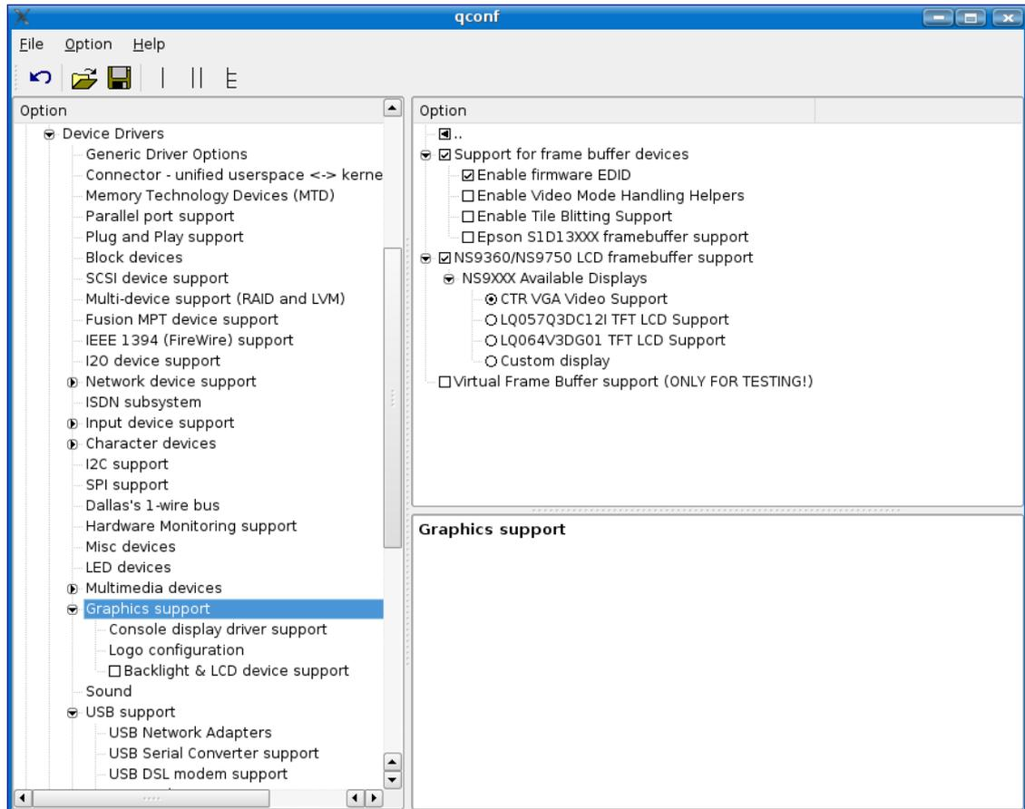
To remove graphics support, uncheck the **NS9360/NS7520 LCD framebuffer support**.
