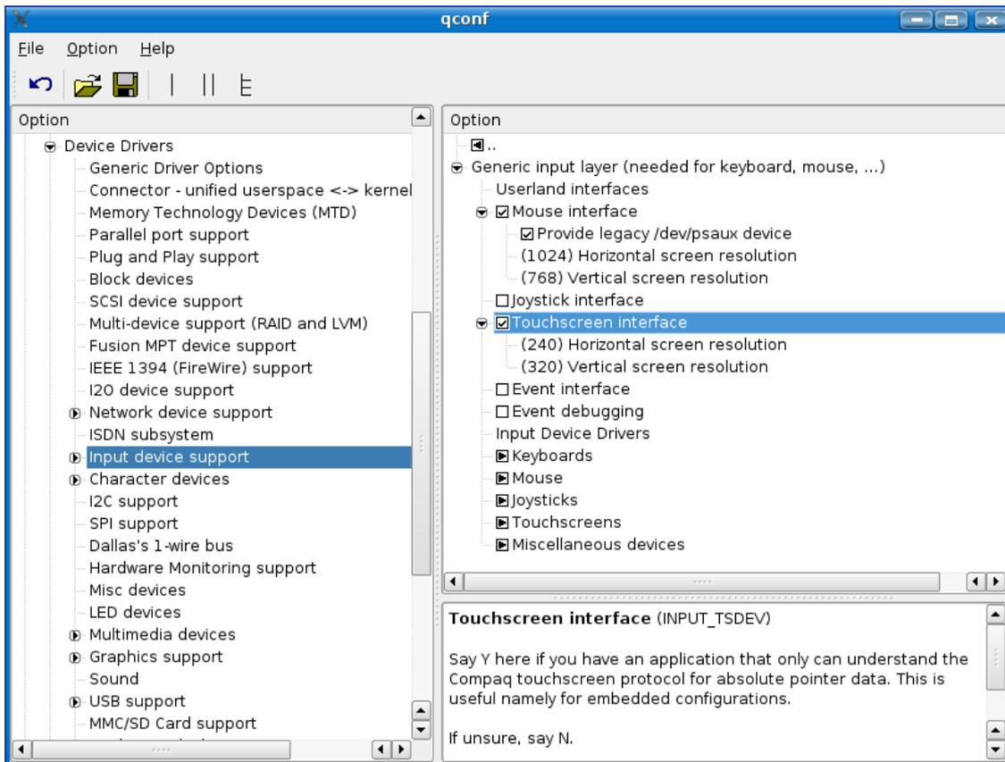
Enable the element **Touchscreen interface**. Then click the **Touchscreens** element and enable **ADS 7846 based touchscreens**.
