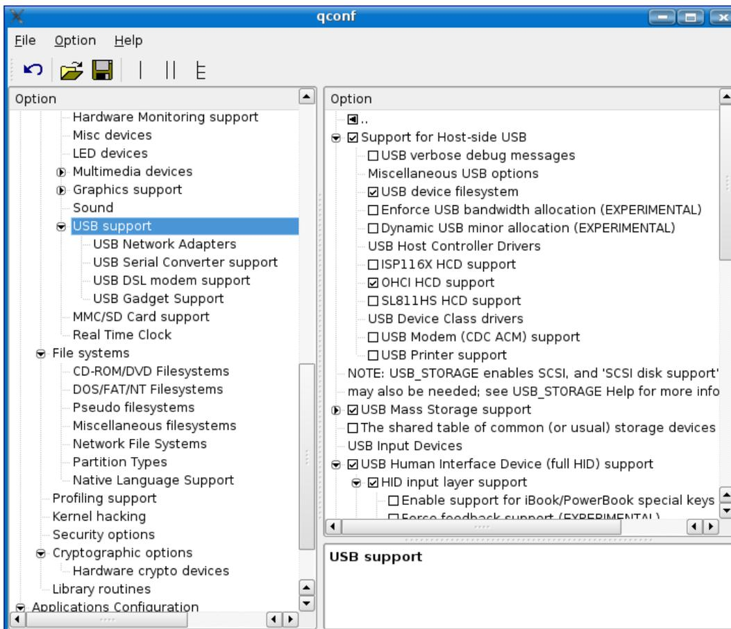
Check whether the items shown in the figure have USB support for storage media, such as USB Flash disks, and for HID input devices, such as a USB mouse.
