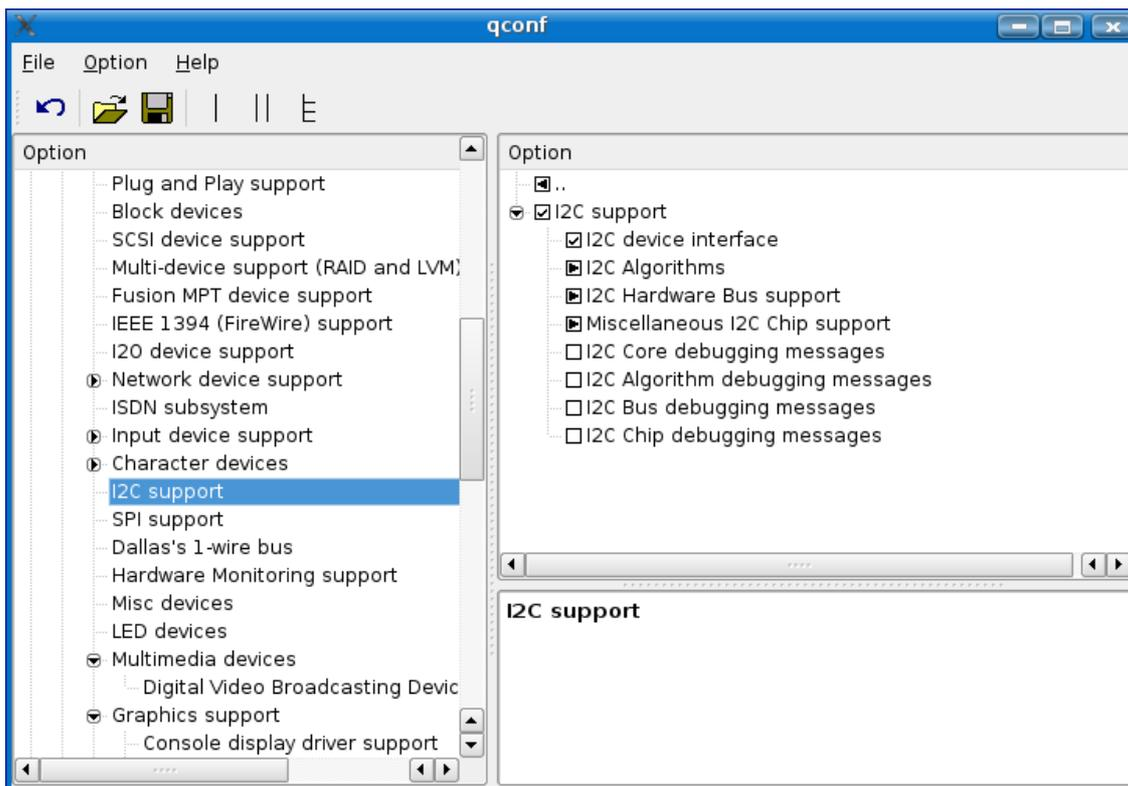
In the displayed configuration information, the following items must be checked for having support for the I<sup>2</sup>C interface and the I<sup>2</sup>C I/O port:
