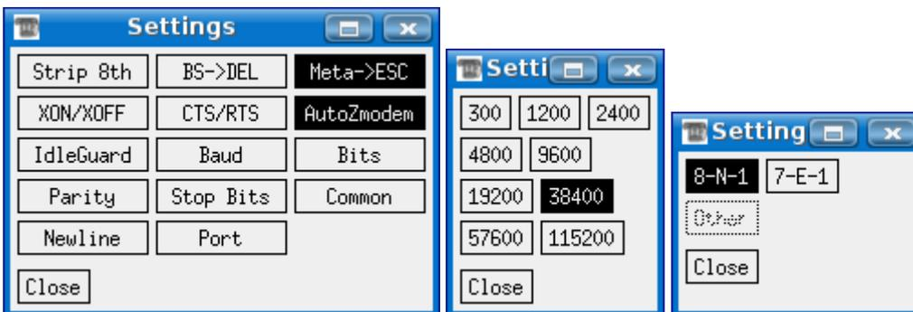
Press the **Baud** button, and select 38400. Press the **common** button, and select 8-N-1.
