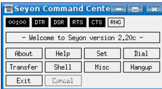
In the **Seyon Command** window, press the **Set** button to open the settings window. In the settings window, the communication parameters can be adjusted.
