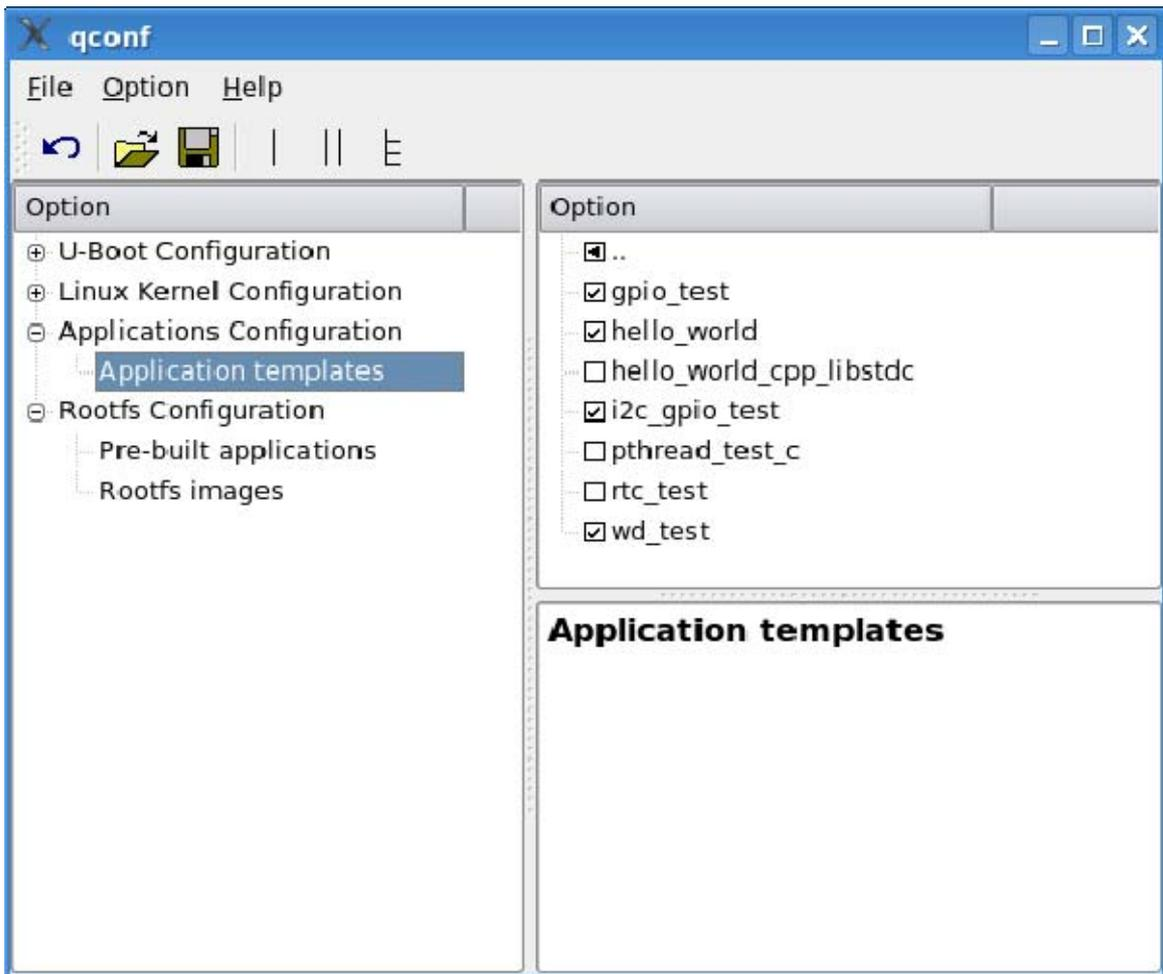
Under **Applications Configuration > User application templates**, select which templates to include in the project. For example, check **gpio\_test** and **hello\_world**, save, and exit the configuration tool.
