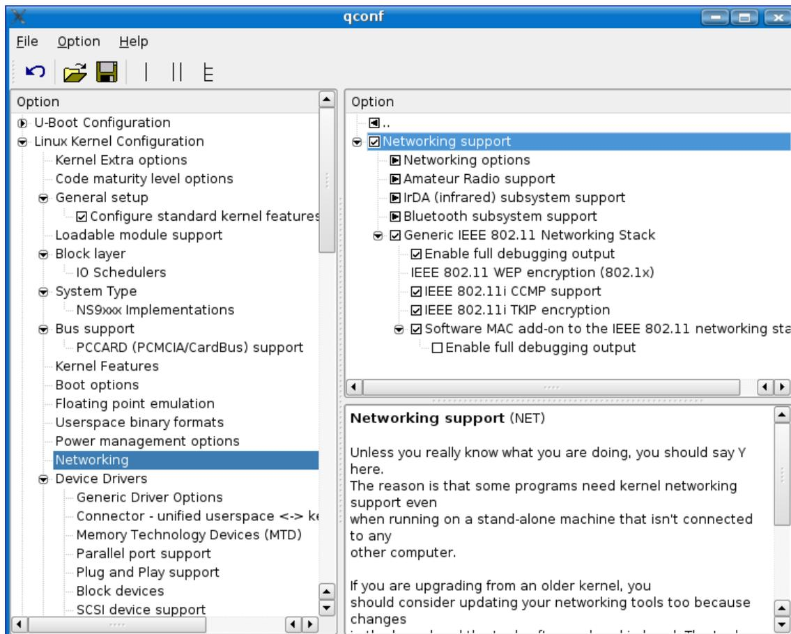
The tool allows customizing the kernel as needed. Most of the options can be built directly into the kernel or as modules (explained in following section).
