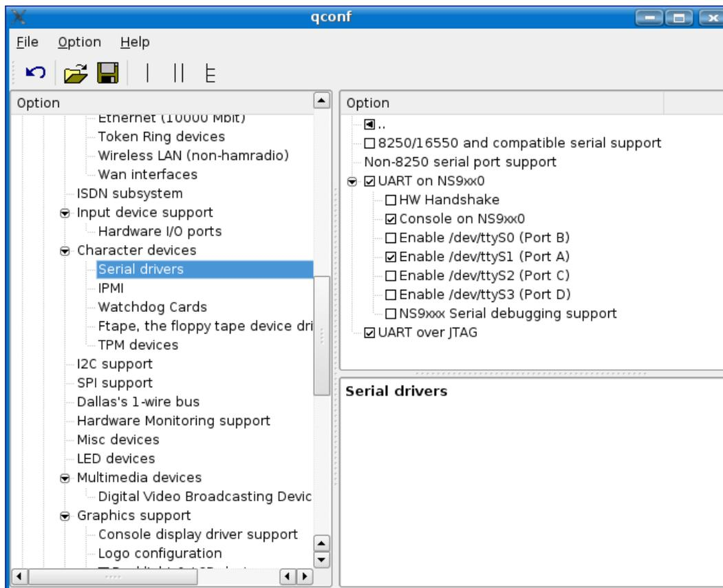
Enabling the element **UART on NS9xx0** grants access to enabling each of the four serial ports in UART mode.
