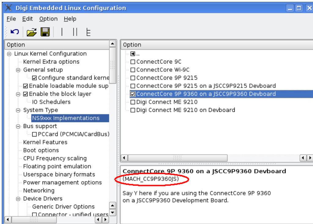
The code in the file *mach-cc9p9360js.c* is specific to the ConnectCore™ 9P 9360 (CC9P9360) module running on the Digi JSCC9P9360 development board. By selecting this machine, the kernel will add support for the specific hardware contained in that module and development board.
