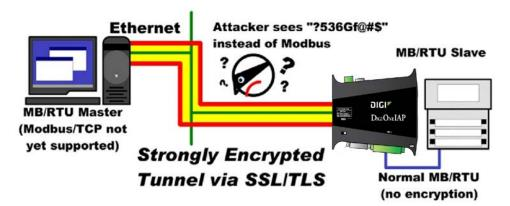
The TCP/IP stack in the Digi One IAP supports SSL v3.0 and TLS v1.0 (also called SSL v3.1). Its preferred ciphers are the US government-promoted 128-bit or 256-bit AES ciphers. It also supports the older 3DES cipher, but this should not be used if AES is available, since it is much more CPU intensive.
