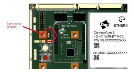
b. If using an SBC version2 (30014752-02), set the boot source microswitches: SW3.1: OFF, SW3.2: ON.
