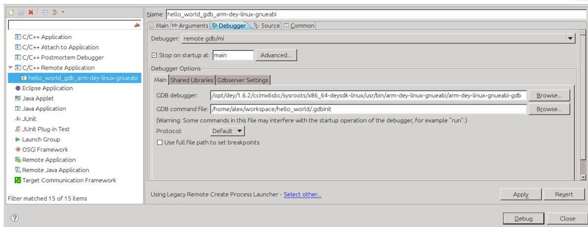
3. Click the Debug button. The debug perspective appears with the application executed on the external hardware.
