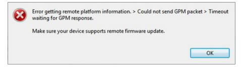
Your remote radio module probably does not support remote firmware update. The following radio modules support the remote firmware update feature:
