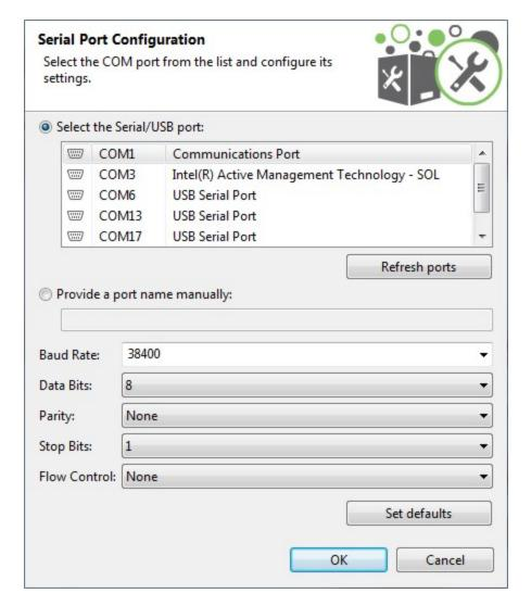
2. Select the device's serial port, or provide it manually. The rest of the parameters are loaded with their default values.
