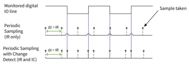
**Note** Use caution when combining Change Detect sampling with sleep modes. **IC** only causes a sample to be generated if the change takes place during a wake period. If the device is sleeping when the digital input transition occurs, then no change is detected and an I/O sample is not generated. Use **IR** in conjunction with **IC** in this instance, since **IR** generates an I/O sample upon wakeup and ensures that the change is properly observed.
