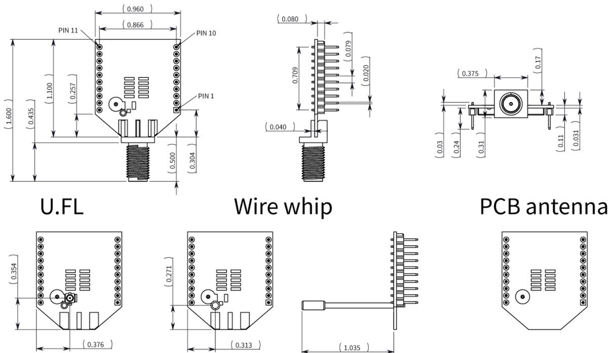
The drawings below show the XBee-PRO through-hole model.
