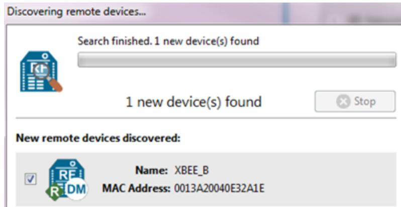
When the discovery process is finished, XCTU lists discovered devices found within the network in the **Discovering remote devices** dialog.
