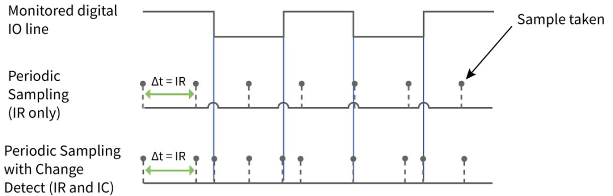
Enabling edge detection forces an immediate sample of all monitored digital I/O lines if any digital I/O lines change state.
