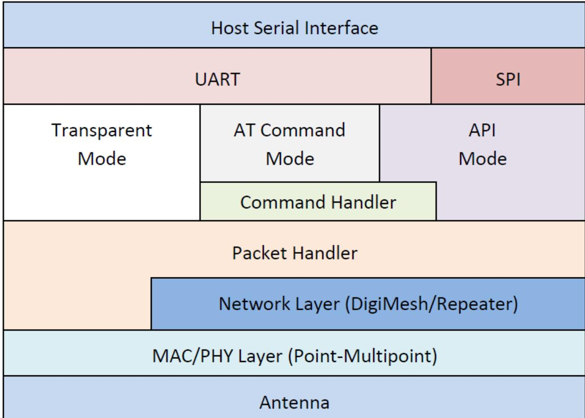
The command handler code processes commands from AT Command Mode or API Mode; see [AT commands](#). The command handler also processes commands from remote devices; see [API frame exchanges](#).
