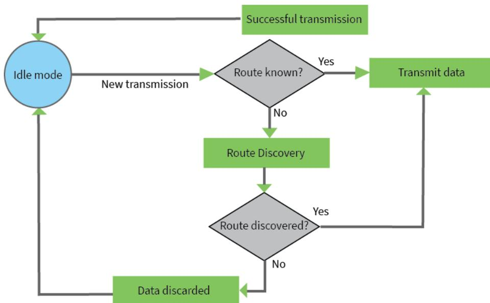
When DigiMesh data is transmitted from one node to another, the destination node transmits a network-level acknowledgment back across the established route to the source node. This acknowledgment packet indicates to the source node that the destination node received the data packet. If the source node does not receive a network acknowledgment, it retransmits the data.
