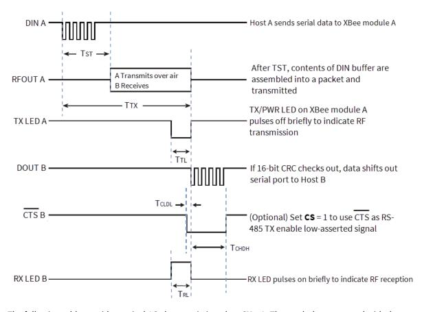
The following table provides typical AC characteristics when  $\mathbf{SY} = 0$ . The symbols correspond with the previous two figures.
