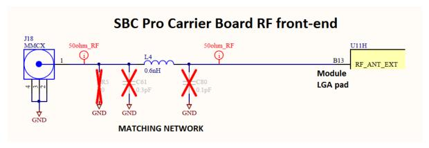
The RF output power at the U.FL connector has been calibrated based on its current matching network. Via stored tables on the firmware, a flat RF output power over frequency is provided at the U.FL connector. (That is, the same amount of power is delivered at each frequency over the band.)
