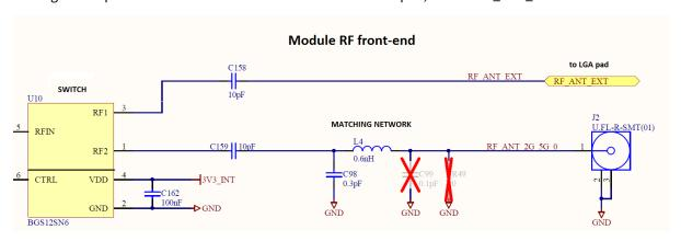
The RF\_ANT\_EXT comes directly (AC coupled by a cap) from the digital switch because the matching network implemented at the RF path for the U.FL connector is not present. Instead, it is assumed that this matching network will be located on the carrier board to compensate for the mismatching introduced when routing from the LGA pad to the carrier board.
