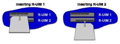
In both cases, the end of the R-UIM card with the chamfered corner should be inserted first. For R-UIM 1 the contacts should be face down. For R-UIM 2 the contacts should be face up.
