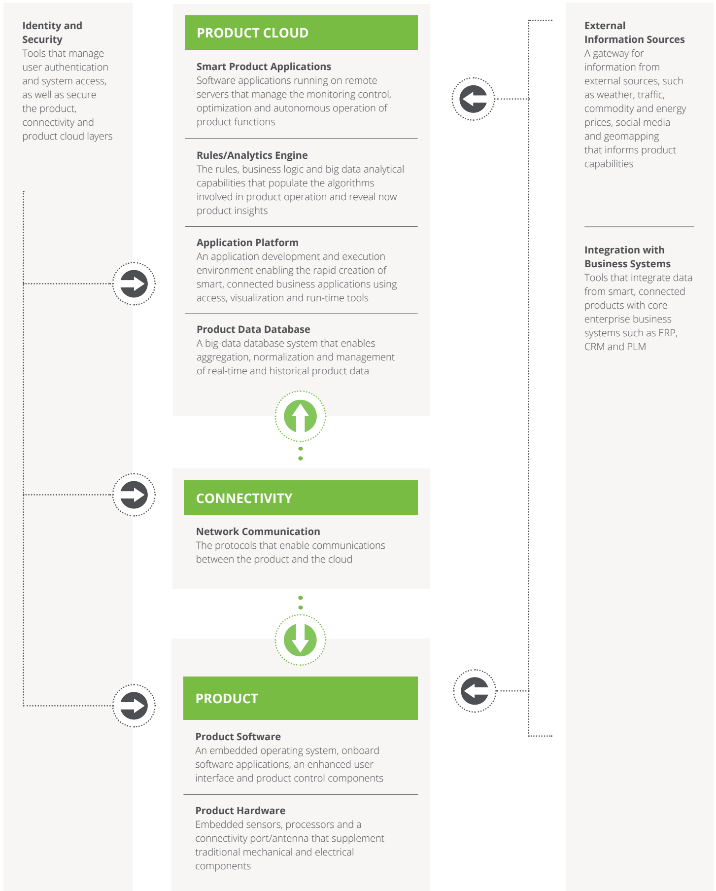
FIGURE 1: SMART IOT ARCHITECTURE
